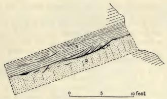
Fig. 12.—Great Gulch mine, Silver Peak, Nevada. Longitudinal vertical section of mine incline, following gold quartz vein (Q) in schist (S), with auriferous arsenopyrite (M) subsequent to the quartz, in the hanging wall of the vein. This position indicates ascending solutions. After J. E. Spurr: Professional Paper 55, U. S. Geol. Surv.; Fig. 17.
